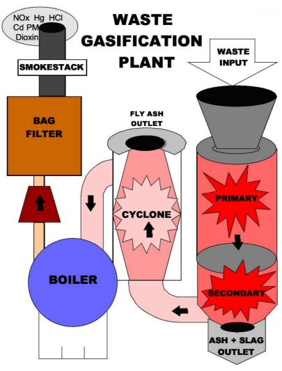
Figure 1: Diagram of the Waste Gasification Process
