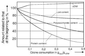
Figure 3.6 Change of the sewage sludge matrix due to partial oxidation by ozone.
