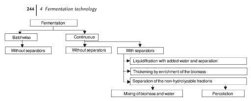
Figure 4.1 Overview of different processes to produce biogas.
