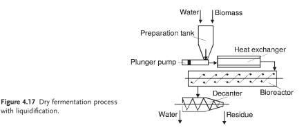
A jacketed tube, through which the moistened biomass is slowly pushed with a residence time of approximately 1 day, serves as a heat exchanger. It is heated with hot water. The subsequent fermentation takes place in a horizontal bioreactor with a flow-through process. The reactor consists either of steel or of concrete coated on the inside with a thin steel panel lining material. After fermentation, dehydration is performed on belt-type presses, filter presses, or decanters (Figure 4.18).
