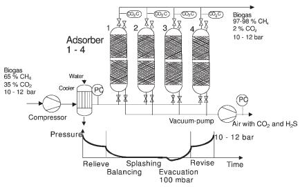
Figure 3.6 Adsorption plant with pressure swing technology.
