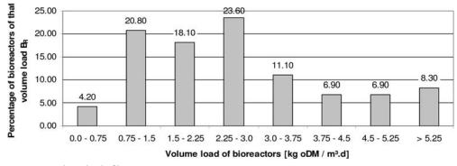
Figure 4.5 Volume load of bioreactors.
