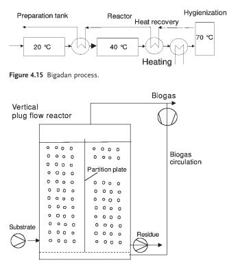
Figure 4.16 Valorga-biogas plant.
