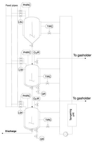
Figure 3.2 Piping instrumentation diagram of a pilot plant.<sup>52)</sup>
