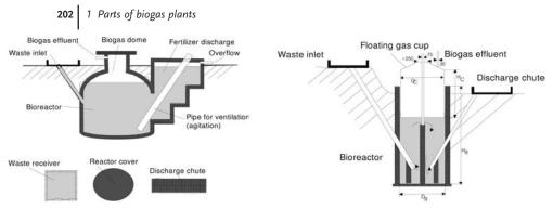
Figure 1.2 Bricked tank: Gasdome (left), Floating cup (right).
