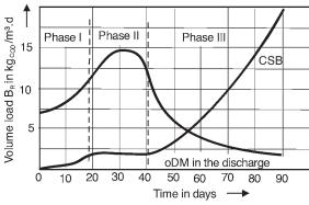
Figure 4.31 Starting phases of a UASB-reactor.
