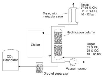
Figure 3.7 Gas liquefication plant in Aklam (Netherlands) with deep-temperature rectification.
