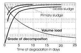
**Figure 4.25** Volume load and grade of decomposition for different sewage sludges depending on the time of degradation at mesophilic conditions.
