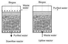
Figure 4.34 Technologies of fixed-bed reactor.
