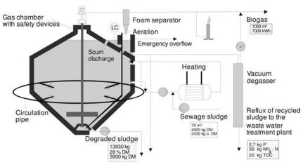
Figure 4.21 Single-stage sewage sludge fermentation plant with internal phase separation.
