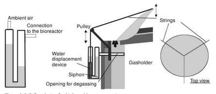
**Figure 1.6** Safety device for high and low pressure in an agricultural plant: U-tube (left), Bioguard<sup>TM</sup> (right).
