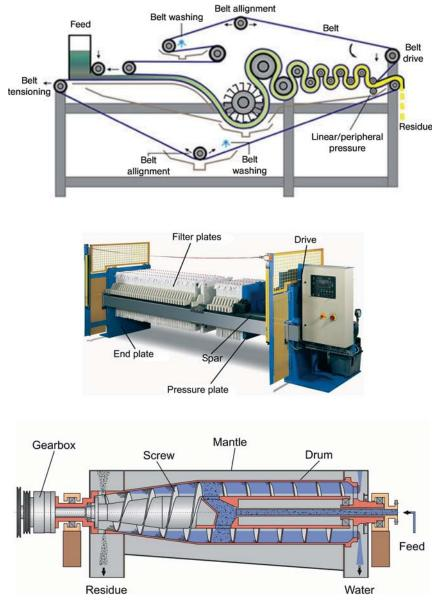
Figure 4.18 Principle of a belt-type press (above), filter press (middle), and decanter (below).
