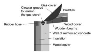
Figure 4.6 Components of a gas-tight cover for a bioreactor.
