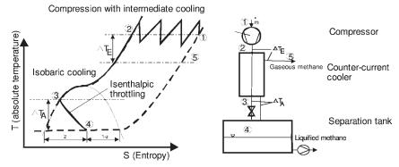
Figure 4.1 Thermodynamic process of gas liquefaction.
