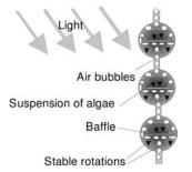
Figure 2.9 Reactor for micro-algae growth.
