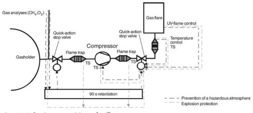
Figure 1.5 Safety devices around the gas flare.<sup>20)</sup>
