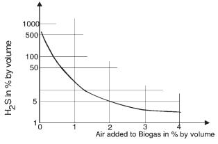
**Figure 3.1** Correlation between hydrogen sulfide content in biogas and air flow into the bioreactor.
