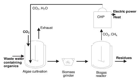
Figure 2.5 Biogas reactor plant based on cultivation micro-algae.
