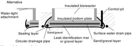
Figure 4.7 Drainage of a bioreactor.
