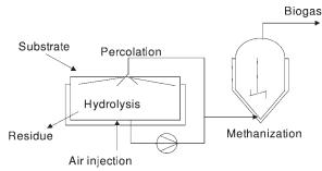
Figure 4.46 Prethane<sup>™</sup>/Rudad<sup>™</sup>-Biopaq<sup>™</sup> process.
