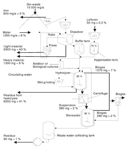
Figure 4.41 Two-stage biogas production plant for bio waste.
