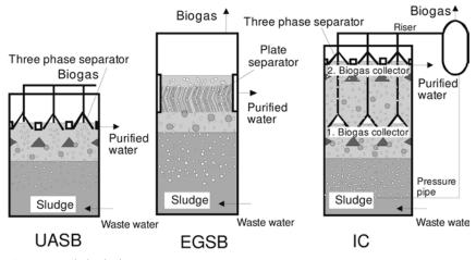
Figure 4.29 Sludge-bed reactors.
