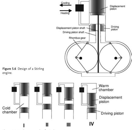
Figure 5.7 Working principle of a Stirling engine.
