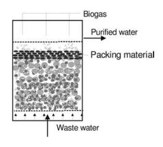
Figure 4.38 CASB-reactor.
