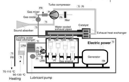
Figure 5.4 CHP instruments.
