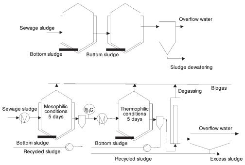
Figure 4.22 Process with multistage fermentation.
