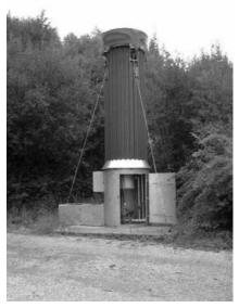
Figure 2.2 Gas flare for high temperature (1050°C) with hidden flame.
