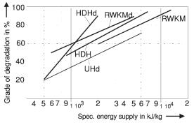
**Figure 3.3** Comparison of different processes for the mechanical disintegration of sewage sludge (UHd = Supersonic with pre-thickening to abt. 40g/kg; HDH d = High pressure ho-mogenization with pre-thickening to abt. 40g/kg; HDH = Homogenization at abt. 10g/kg; RWKM d = Agitation with ball mill with pre-thickening at abt. 40g/kg; RWKM = Agitation with bal mill at abt. 10g/kg.
