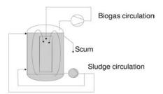
Figure 4.40 Loop reactor.
