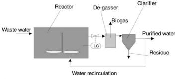
Figure 4.36 Contact process.
