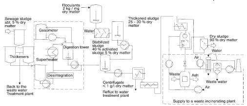
Figure 2.4 Sewage sludge treatment plant<sup>31)</sup>
