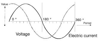
Figure 5.2 Phase difference between electric current and voltage.
