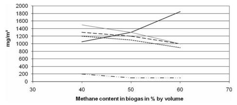
$\label{eq:Figure 5.15} \begin{array}{l} \mbox{Impurities in the exhaust gas of a CHP at different} \\ \mbox{methane contents (----) NO}_{x; \ (----) \ Formaldehyde; \ (----) \ Total-carbon; \ (----) \ Methane \ loss; \ (----) \ CO. \end{array}$
