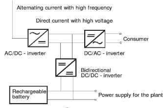
Figure 5.14 Electronic gear.49)
