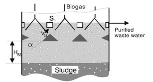
Figure 4.30 Three-phase separator in a UASB-reactor.
