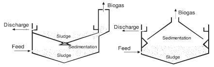
Figure 4.28 Common anaerobic sewage treatment plants:<sup>75)</sup> Clarigester (left), UASB-reactor (right).
