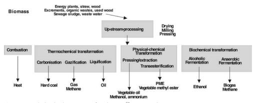
Figure 2.2 Applied technologies to transform biomass<sup>11)</sup> into secondary energy sources.
