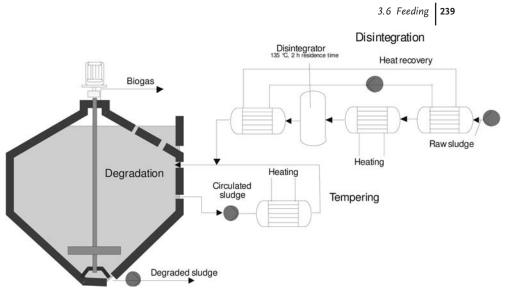
**Figure 3.7** Flow diagram of a thermal disintegration process with indirect heat exchange and water circulation.
