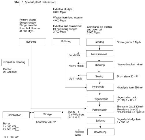
Figure 5.1 Biogas plant in Radeberg (Germany).94)
