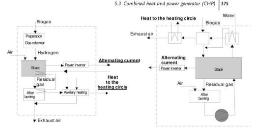
Figure 5.10 Flow chart of fuel cell plants: PAFC (left); MCFC (right).
