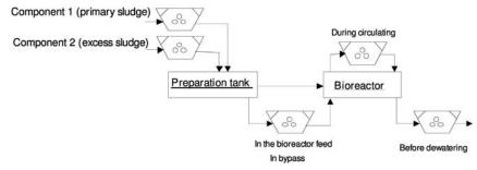
Figure 3.2 Recommended stages for the disintegration process.
