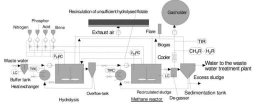
Figure 4.39 Two-stage bioreactor plant for industrial waste water.
