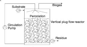
Figure 4.47 Dry anaerobic composting process.
