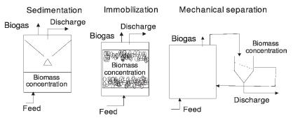
Figure 4.27 Technical alternatives for phase separation.
