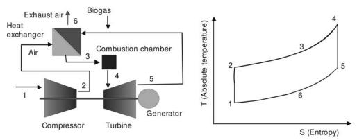
Micro gas-turbines are regulated only by varying the fuel supply.
