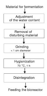
Bio wastes (market waste, leftovers, wastes from households) are to be fermented under dry more than 15% DM or liquefied (less than 15% DM) conditions. Wet fermentation is much more frequently used than dry fermentation. Sometimes special procedures such as percolation or squeezing-off procedures are used for the separation of a fermentable liquid (pressing water, extraction water) or a compostable residue.
