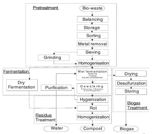
Figure 5.2 Basic flow sheet of a combined wet and dry fermentation process of bio waste.98)
