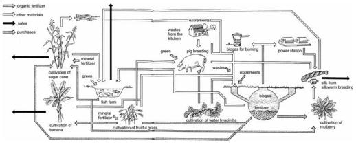
Figure 4.2 Autarc system in developing countries.
