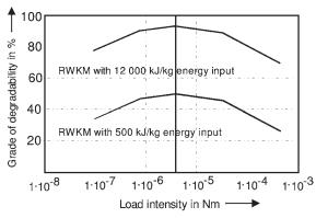
**Figure 3.5** Influence of the load intensity on the grade of degradation at constant specific energy (RWKM = agitated ball mill).
