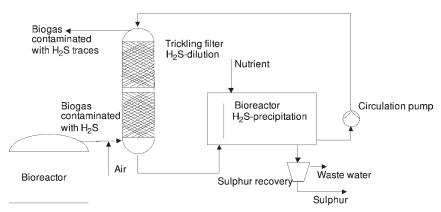
Figure 3.2 Trickling filter plant with separate bioreactor.
